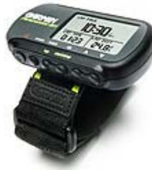
The ForeRunner contains a Lithium Ion battery that can run the unit for 14-16 hours. A charging unit is provided – with recharging taking 1-2 hours.
